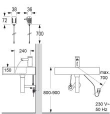
lino lavatory faucet L30, with IR sensor, with temperature-mixing, low pressure (for open water heater), chromed
