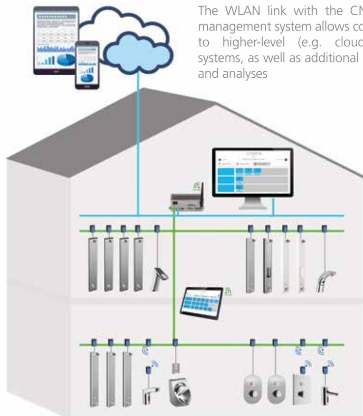
The WLAN link with the CNX water management system allows connection to higher-level (e.g. cloud based) systems, as well as additional functions and analyses
