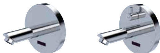
WV20 / WV10 (flush mounted) with IR sensor with / without temperature control Projection: 120/170/220 mm, chrome plated
