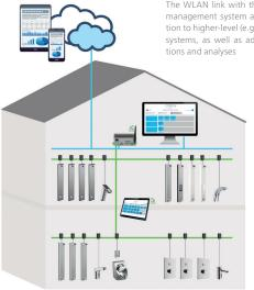
The WLAN link with the CNX water management system allows connection to higher-level (e.g. cloud based) systems, as well as additional func-
