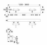
lino multiple washing system W35, with IR sensor, with thermostat, chromed
