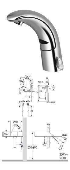
iQ lavatory faucet A30, with IR sensor, pressureless (for open water heater), with temperature-mixing, chromed
