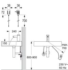
lino lavatory faucet L30, with IR sensor, with temperature-mixing, low pressure (for open water heater), chromed
